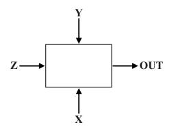
The output at **OUT** is the same as the input signal at **X** when the input signal at **Z** is 0. The output at **OUT** is the same as the input signal at **Y** when the input signal at **Z** is 1.
